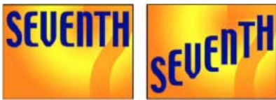
Original (left) and after selecting the entire word, setting Based On to Characters, animating the y Position value so that the word is at the bottom of the frame, and setting Shape to Ramp Down (right)
